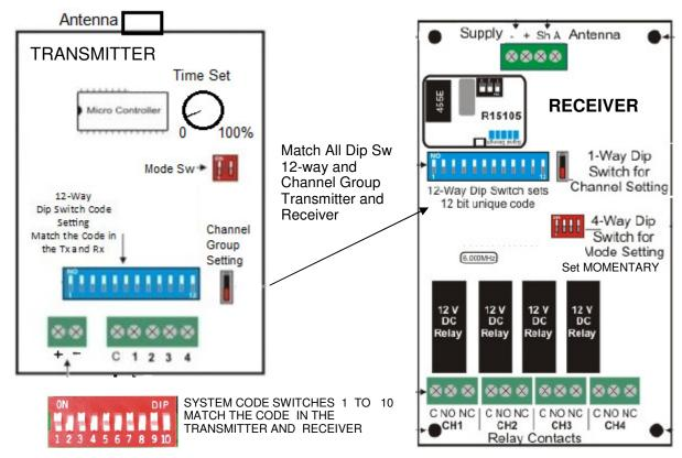
NOTE: Transmitter and receiver antennas shall be mounted facing the same vertical position, (same polarity pattern ) even when there is no line of sight.
