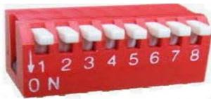
DIP Switch setting 1 to 4 match TX to RX, Factory set 1234 ON
