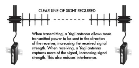
Make sure Yagis are phased (oriented) correctly with respect to each other.
